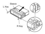
4. Mount the sleeve by inserting the sleeve into the opening of the dashboard and bend open the tabs located around the sleeve with a screwdriver. Not all tabs will be able to make contact, so examine which ones will be most effective. Bend open the appropriate tabs behind the dashboard to secure the sleeve in place.
